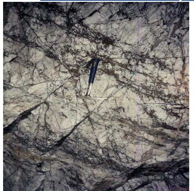
This is a picture of the vein in an underground stope, showing sulfides and gold in white quartz.
