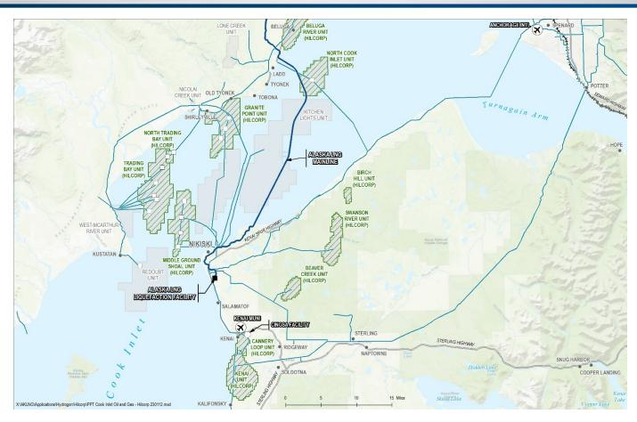
The Alaska Department of Natural Resources identified that Cook Inlet Basin has the highest  $CO_2$  storage potential in Alaska with an estimated 50 GT in depleted reservoirs, saline aquifers, and coal beds. A transmission pipeline(s) from the  $CO_2$  sources at Nikiski can deliver  $CO_2$  to one or more of the  $CO_2$  sequestration fields in Cook Inlet, including the Kenai Gas Field.
