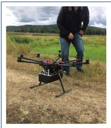
Multi-rotor UAS outfitted with in-situ gas detection sensor
