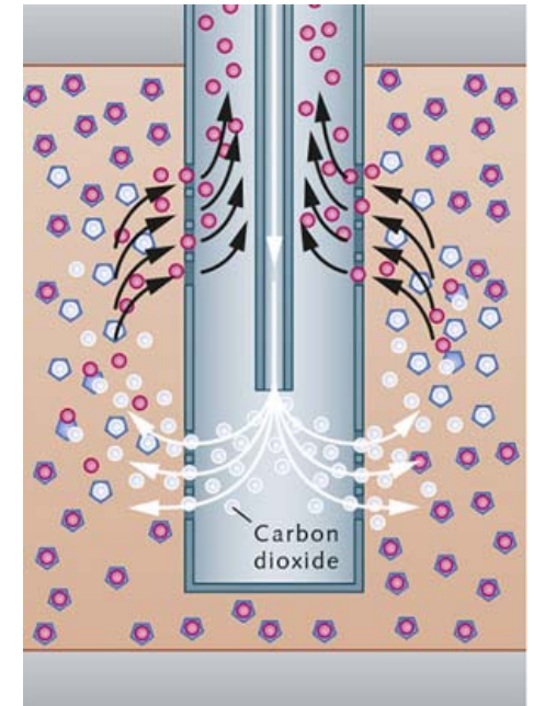
Scheme showing the process of pumping in high pressure CO 2 to extract trapped methane and other gas hydrates.
